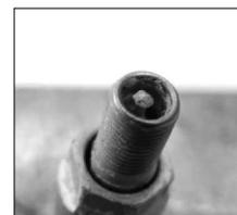
**Unplated valve core, corroded in stem (valve core will not actuate)**
