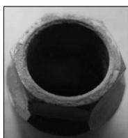
**Corroded nut will not torque to specified torque**
